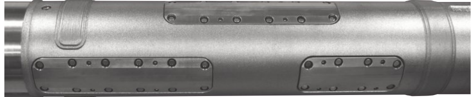
Control Electronics Hatches
