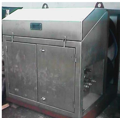
ESD CONTROL PANEL
