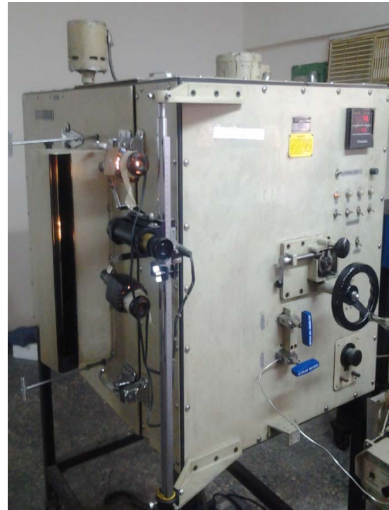
CONDENSATE/VOLATILE OIL CELL
