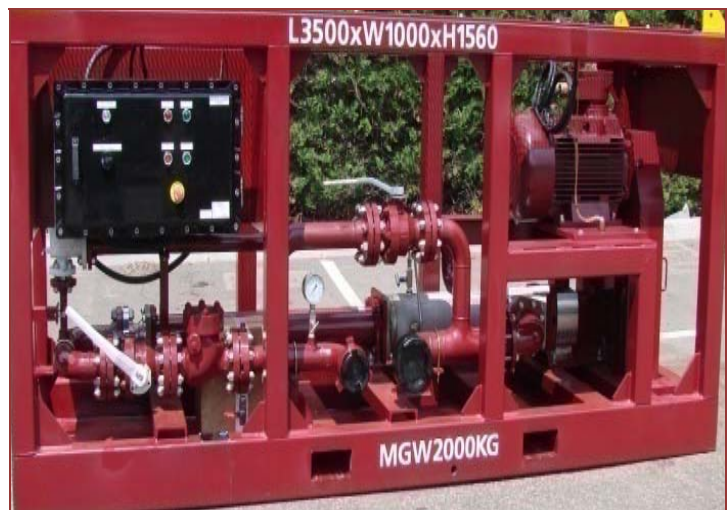
CRUDE OIL TRANSFER CENTRIFUGAL PUMP
