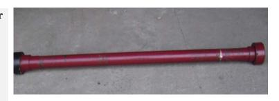
Its presence prevents the loss of valuable wire line tools in case the rope socket is accidentally stripped off. Any tools dropped down the lubricator will be caught by the slotted Stop in the Tool Trap. The Stop has an opening larger than the wire line, but smaller than the subsurface tools.
